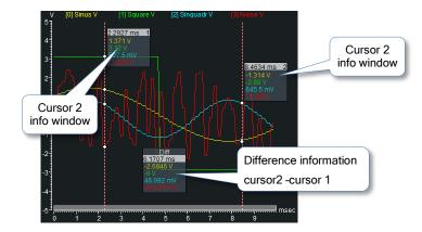
The cursor difference window shows in the first line the time or frequency span between the first two cursors. The following lines show the difference of the signal values displayed in cursor window one and two. For time diagram you can switch the difference window to another mode where it shows the rms value between the first two cursors. To change the difference calculation method tap on the cursor difference window and choose on the appearing context menu between these entries:
